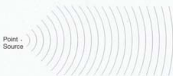
Figure 0.12. Spherical waves propagating outward from the point source. Far from the point source, the radius of the wavefront is large and the wavefronts approximate plane waves.
